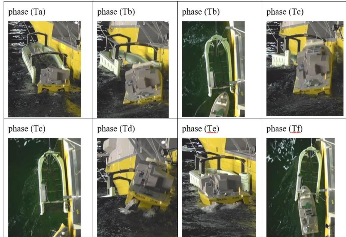
Example of recovery test (head seas, 5 kts, Hs=4m (SS6))
