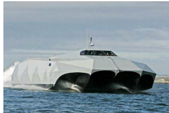
Figure 24 : Coque du Stiletto.
